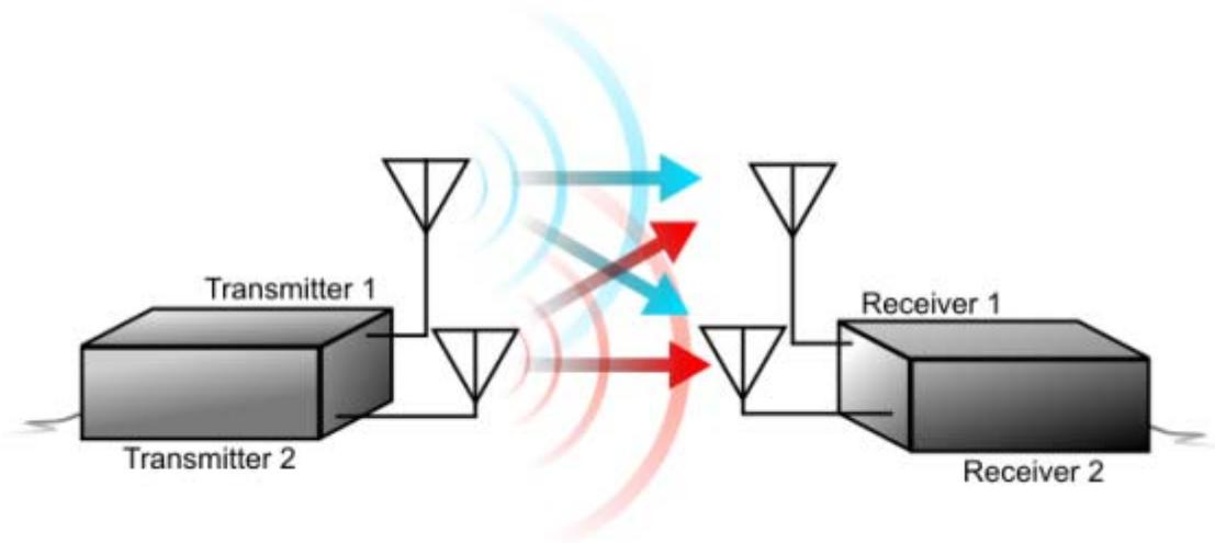
d. MIMO uses multiple transmitters, receivers and antennas to send multiple signals over the same channel, multiplying spectral efficiency.
