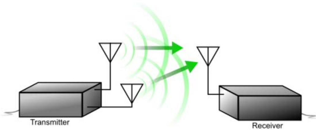
a. Beamforming (beam steering) employs two transmit antennas to deliver the best multipath signal
