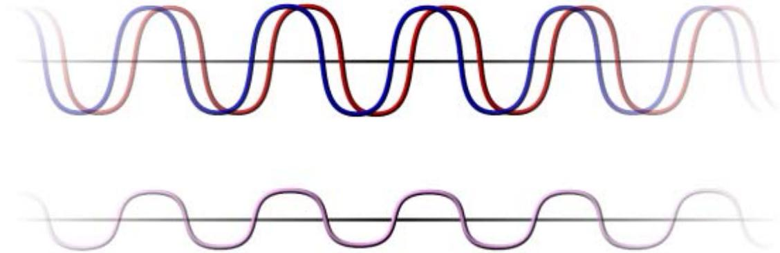
b. Multipath signals arriving slightly out-of-phase combine at the receiver to create a somewhat weaker and less distinct signal
