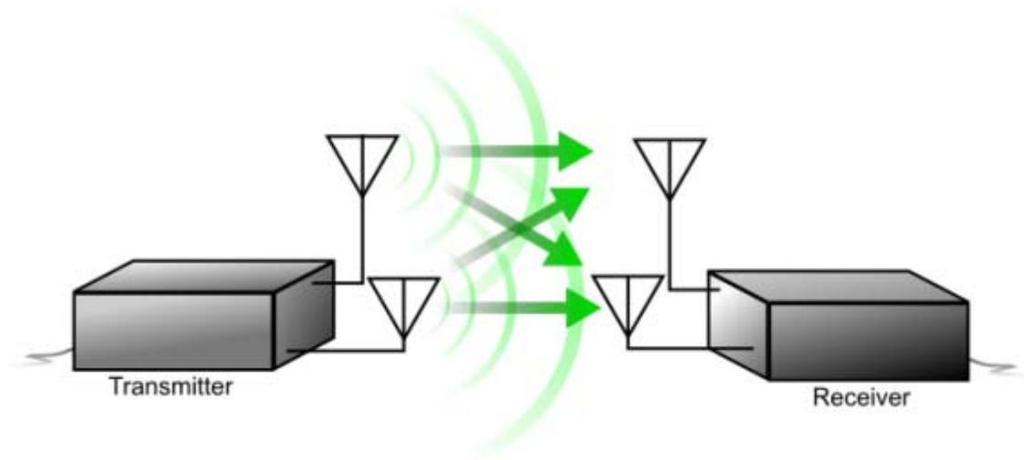
c. There may be a physical resemblance between radio systems using a combination of beam steering and diversity and MIMO systems. Note, however, that with the beam steering/diversity approach, only one signal is sent over the channel.
