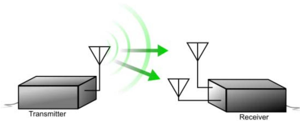
b. Diversity (receive combining) uses two receive antennas to capture the best multipath signal
